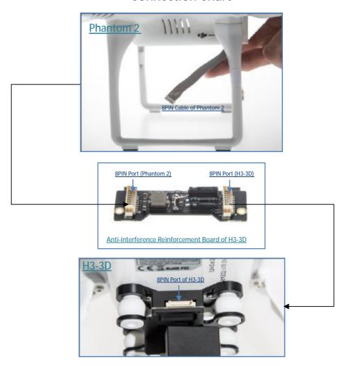
The Anti-interference Reinforcement Board is an accessory of the DJI H3-3D (For Phantom 2 Only version), you may follow the connection chart above to connect the Phantom 2 and H3-3D with the board. Please pay attention to the Input and Output ports of the board. There are two ways to mount the board, you can use a 3M double-side tape to fix it at the bottom of the Phantom 2, OR you can mount the board directly inside the Phantom 2 as shown in the picture below.
