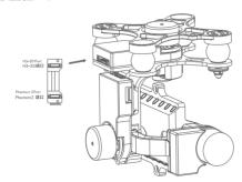
\* 8-pin port on the H3-3D gimbal should only be used for connecting to the Phantom 2. Do not connect other devices (such as a video downlink transmitter) to this port, otherwise the gimbal may be damaged. 云台上的8针端口只用于通过标配的8针线连接到Phantom 2。禁止将其它配件(如5.8G图传发射机)连接到此端口,否则会引起云台数值。
