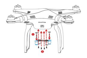
Attach the bottom plate of damping unit to the upper plate of the damping unit through four vibration absorbers. Be sure the lip of the vibration absorbers are properly inserted through the mounting holes of the bottom plate.
