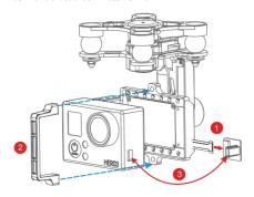
\* Do not power on the aircraft before mounting the camera onto the H3-3D gimbal, otherwise the gimbal may be damaged.
