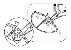
Only use the Prop Guard screws when Prop Guards are mounted to avoid loose joints or damage to the motors.
