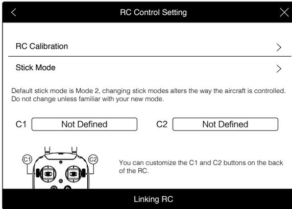
4. The remote controller is ready to link. The Remote Controller Status Indicator blinks blue and a beep is emitted.
