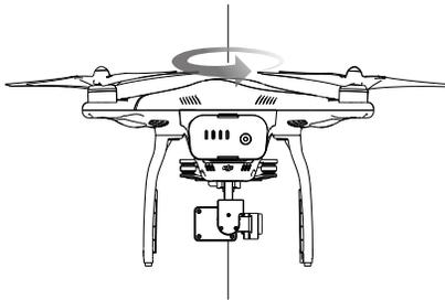
3. Hold the aircraft vertically, with nose pointing downward, and rotate it 360 degrees around the center axis. Recalibrate the compass if the Aircraft Status Indicator glows solid red.
