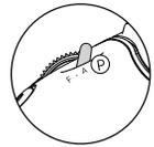
**⚠** The performance of your Vision Positioning System is affected by the surface over which it is flying. The ultrasonic sensors may not be able to accurately measure distances when operating above sound-absorbing materials. In addition, the camera may not function correctly in suboptimal environments. The aircraft will switch from P-mode to A-mode automatically if neither GPS nor Vision Positioning System are available. Operate the aircraft with great caution in the following situations:
