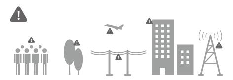
Avoid flying over or near obstacles, crowds, high voltage power lines, trees or bodies of water. DO NOT fly near strong electromagnetic sources such as power lines and base stations as it may affect the onboard compass.
