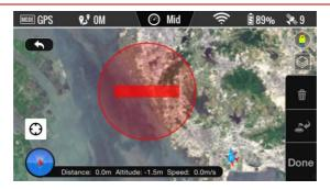
Tap on a waypoint to open a waypoint properties window. Modify longitude and latitude value from the input box. Slide the white dot right to adjust waypoint altitude. The default altitude is set to 98 feet (20 m) and can be adjusted from 0 to 650 feet (200 m). Tap "OK" to save waypoint settings. To delete current waypoint, tap ...
