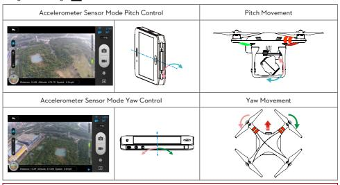
In Accelerometer Sensor Mode, the pitch angle indicator will show a grey area. When the green pitch indicator is inside the grey area, the camera will move according to pitch gestures. When the indicator reaches the boundary of the grey area, pitch gestures will control the camera's pitch speed at a constant rate.
