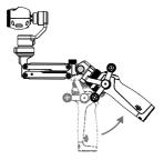
▲ DO NOT attempt to adjust the grip angle without pressing the pivot release button as this will damage the Z-Axis.
