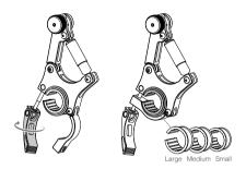
Attach the clamp around your bike's handle bar and tighten the lever to secure. Ensure the vibration damper is perpendicular to the ground to attain optimal stabilization.
