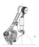
Attach the Osmo handle to the Bike Mount's rosette mount and tighten the knob to secure.
