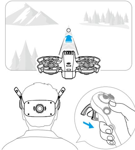
Push the accelerator forward to fly the aircraft in reverse.
