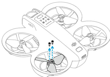
2. Install the marked propellers onto the motors of the marked arms and the unmarked propellers onto the motors of the unmarked arms. Use the screws provided in the packaging to secure the propellers. Make sure to tighten the screws.
