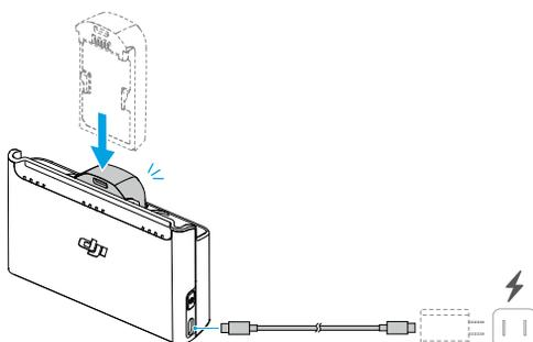
1. Insert the batteries into the battery ports of the charging hub until they click into place.
