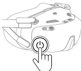
Press the power button once to check the current battery level.
