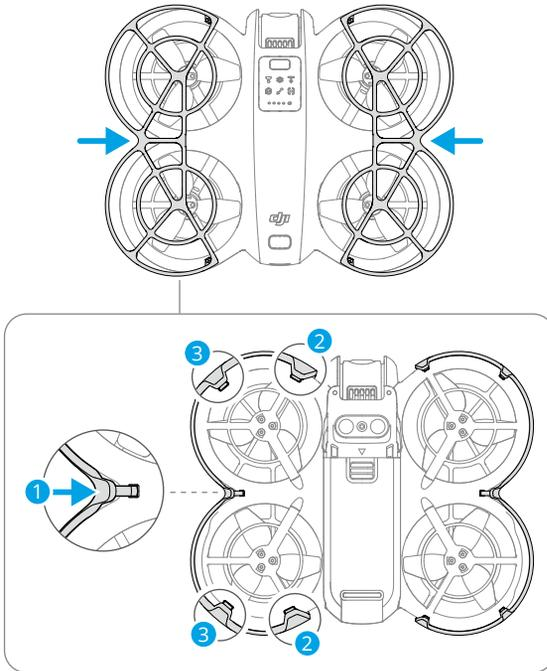
2. Install the other propeller guard in the same way.
