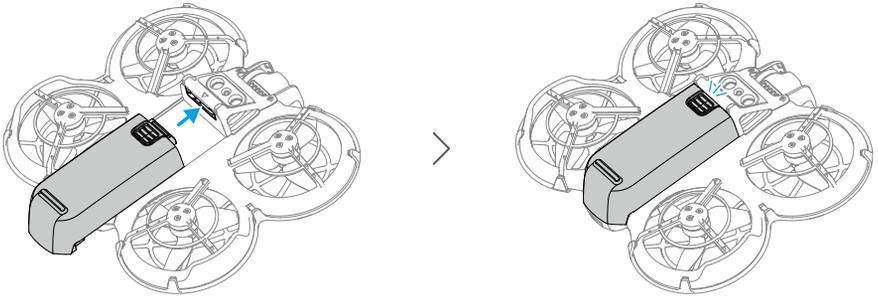
Press the textured part of the battery latch and push the battery to the rear of DJI Neo to remove it.
