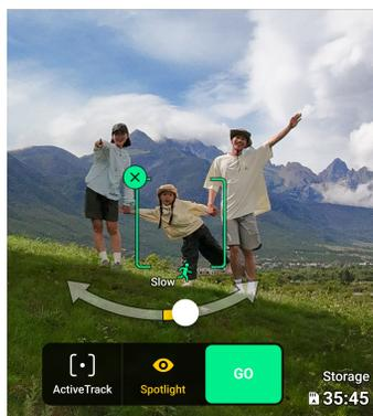
4. Tap on the bottom of the screen to switch to ActiveTrack. Tap **GO** and the aircraft will start tracking the subject automatically. Press the Shutter/Record button on the remote controller or the screen to start taking photos or recording video.
