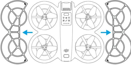
Install the propeller guard by following the steps below.
