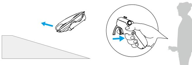
When the aircraft needs to fly at a downward angle, press the accelerator to the second stop while simultaneously tilting the motion controller down.
