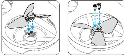
3. Reinstall the propeller guards after installing the propellers.
