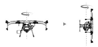
4. The Aircraft Status Indicators show the current flight mode and the calibration page disappears in the app when calibration is complete. If the Aircraft Status Indicators blink red or a calibration failure is displayed in the app, repeat the steps above to calibrate the compass.
