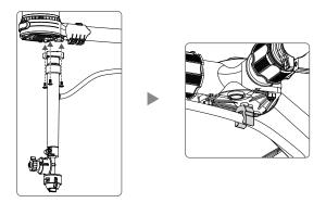
3. Insert the hoses on both sides into the clips on the landing gear.
