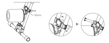
Insert the radar cable into the cable clip on the landing gear leg, then connect it to the radar port on the aircraft body.
