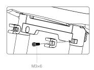
2. Mount the sprinklers with white hoses under motors M3 and M8 (with white circle marks). Mount the sprinklers with black hoses under motors M4 and M7 (with black circle marks). Mount each of the four sprinklers using three M3×8 (Plus) screws, then insert the hoses into the clips at the bottom of the frame arm junctions. Be sure to mount the sprinklers to the mounting holes nearer to the inside of the aircraft, with the hoses facing the frame arm.
