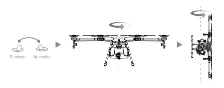
4. The Aircraft Status Indicator shows the current flight mode when calibration is complete. If the Aircraft Status Indicator becomes blinking red, repeat the steps above to recalibrate the compass.
