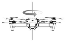
Hold the aircraft vertically, with nose pointing downward, and rotate it 360 degrees around the center axis.
