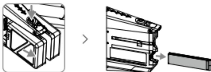
2. Insert the CINESSD into the DJI CINESSD Station, then connect the station to a computer via a USB cable.
