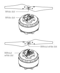
Align the part, labeled A in the diagram below, with the upper side of the securing spring, labeled B, then press the propeller down onto the mounting plate and rotate in the lock direction and until secure.
