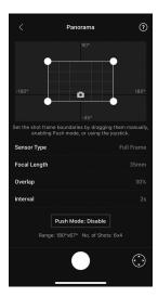
Panorama allows users to capture a series of interconnecting still images with precise control based on the sensor type, lens focal length, overlap, and interval.
