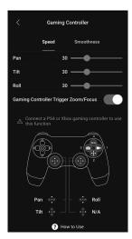
PS4 DualShock and Xbox controllers can be used to control the gimbal and camera. After connecting the controller to the mobile device and gimbal, users can control gimbal movements, focus, and zoom, and can record videos, recenter gimbal, and capture photos.
