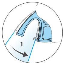
When gently pressing the accelerator to the first stop, you can adjust the aircraft orientation by tilting the motion controller vertically to the left or right.
