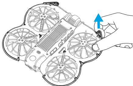
4. Operate along the edge to release the remaining buckles.
