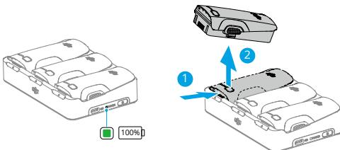
Remove the corresponding battery from the charging hub as shown.
