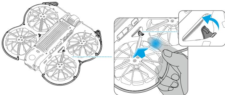
3. Lift the front protrusion of the guard to release the buckle.
