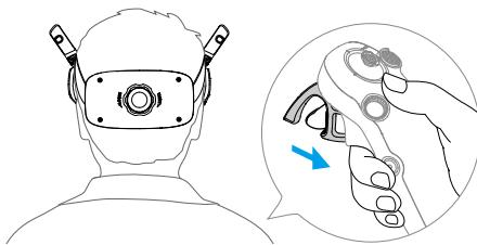
Push the accelerator forward to fly the aircraft in reverse.
