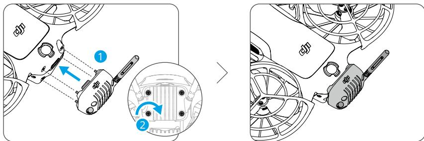
**⚠** • Use the screwdriver provided in the aircraft package to remove and install the screws. Unsuitable screwdrivers may damage the screws.
