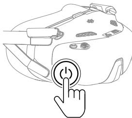
Press the power button once to check the current battery level.
