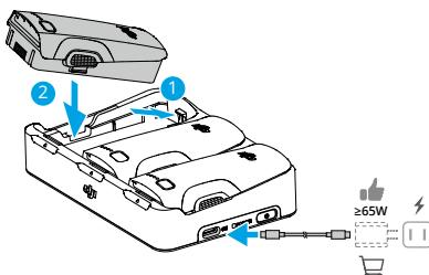
Insert the batteries into the battery ports of the charging hub until they click into place. Connect the charging hub to a power outlet using a USB charger.
