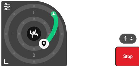
The aircraft will bypass obstacles regardless of the flight modes or obstacle avoidance action settings in DJI Fly when the vision systems are working normally.
