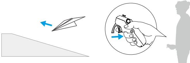
When the aircraft needs to fly at an downward angle, press the accelerator to the second stop while simultaneously tilting the motion controller down.
