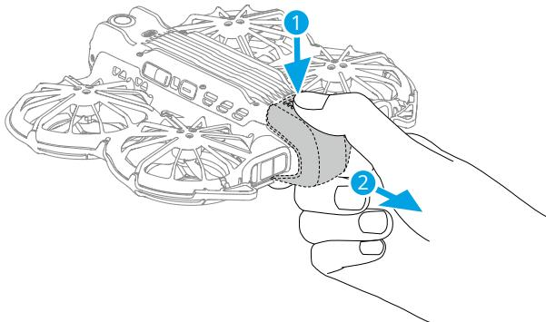
Press, then press and hold the power button to power on DJI Neo 2.
