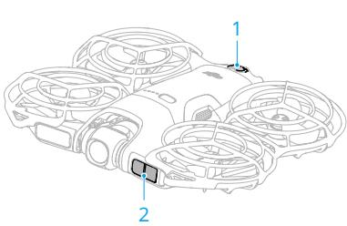
1. Omnidirectional Monocular Vision System
