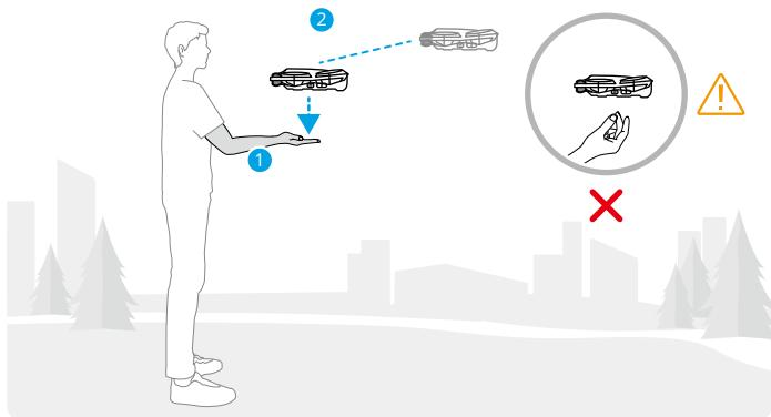
If the aircraft is at a distance, first face the aircraft and extend one arm sideways to signal it to return. After the aircraft flies closer, extend your palm and wait for it to land on your hand.
