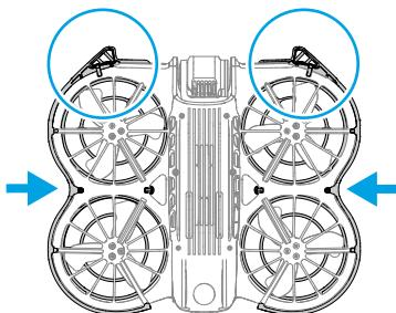
2. Secure all remaining buckles onto the aircraft body to ensure firm installation.
