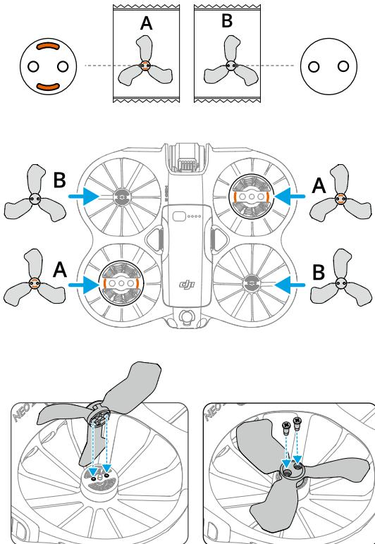
3. Reinstall the propeller guards after installing the propellers.
