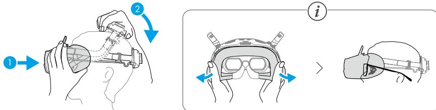
3. Rotate the headband adjustment knob on the battery compartment to adjust the length of the headband.
