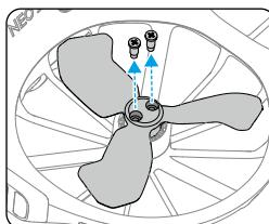
2. Install the marked propellers onto the motors of the marked frame arms and the unmarked propellers onto the motors of the unmarked frame arms. Use the screws provided in the packaging of the propellers to secure the propellers. Make sure to tighten the screws.
