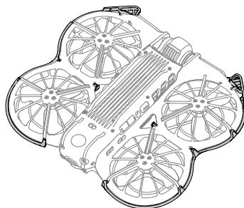
2. Press the center of the guard to release the buckle to open it.
