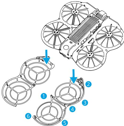
Install the propeller guards by following the steps below.
