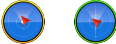
Tap the flight attitude icon to turn on the radar function. Home is located in the center of the radar and the red icon indicates the PHANTOM 2 VISION's current heading, direction, and approximate distance from home. The current longitude and latitude of the aircraft is displayed on the bottom of the radar. Tap the flight attitude icon again to disable the radar.
