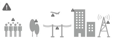
Avoid flying over or near obstacles, crowds, high voltage power lines, trees or bodies of water. DO NOT fly near strong electromagnetic sources such as power lines and base stations as these may affect the onboard compass.
